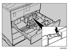
**6** While pressing the release lever, slide the side fences outward.
